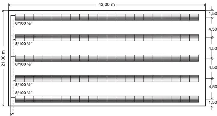
Fig.14 Example of EAE panels in warehouse with average height of 5,5 m and parallel panels on the longest side
